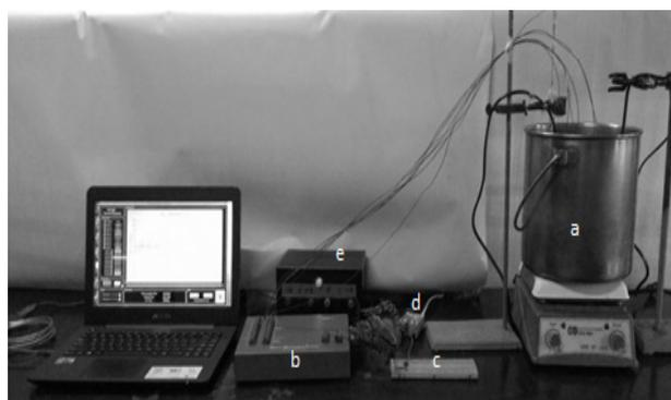
Figure 2. Experimental setup for the pasteurization of guyabano juice. Setup includes (a) water bath, (b) ADC-1, (c) breadboard, (d) relay box, and (e) DC power supply
