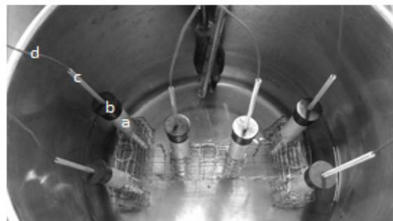
Figure 1. Experimental setup of aluminum tubes in the water bath during guyabano juice pasteurization. Setup includes (a) aluminum tube, (b) rubber stopper, (c) plastic tube, and (d) thermocouple.
